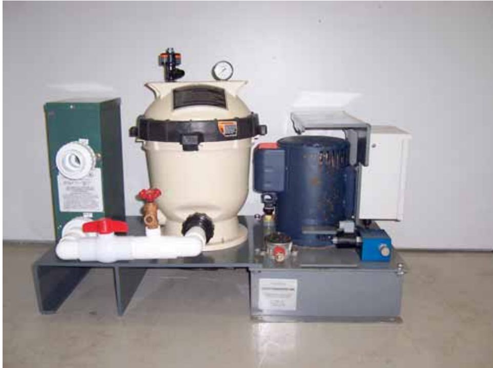
Figure 1: Circulating Pump Foot and PVC Support Base
